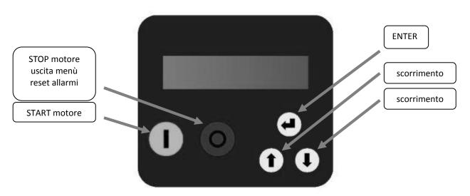
Screen is a back-lit LCD displaying 2 rows of 16 digits each. If the menu indication is longer than 16 digits, the row will scroll
